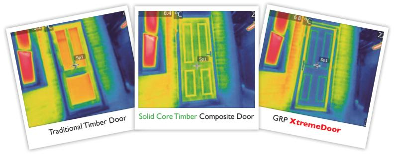
The **XtremeDoor** is **17% more thermally efficient** than a traditional timber door and **19% more thermally efficient** than a composite door manufactured with a timber core.
